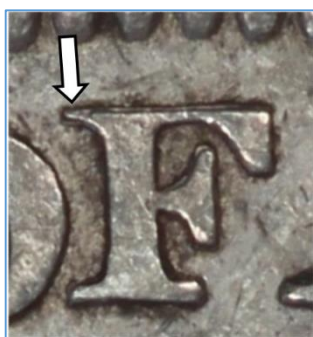
Complete serif (serif repaired on the working hub?)
